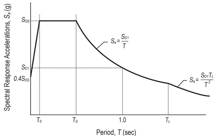
**Figure 4-5.** ASCE 7 design response spectrum showing spectral response acceleration as a function of vibration period.
