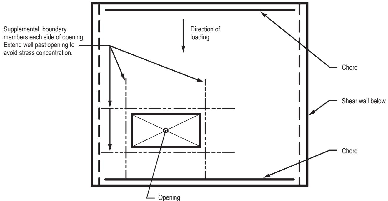
**Figure 3-6.** Wood light-frame diaphragm with opening. Supplemental boundary members are added around the opening.
