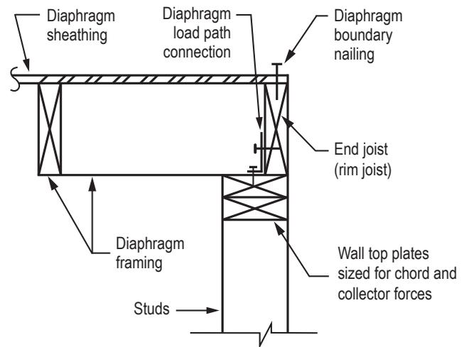
**Figure 3-4.** Wall top plate acting as chord boundary element. The same top plate can also act as the collector boundary element.
