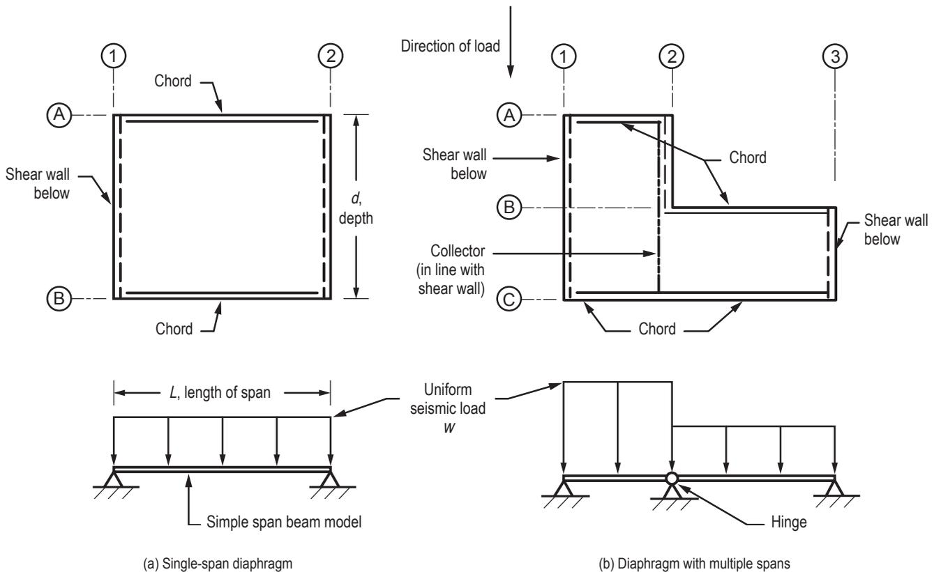
**Figure 3-1.** Plan view of wood light-frame diaphragms.
