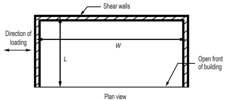
Figure 7-1. Diaphragm in open front structure.
