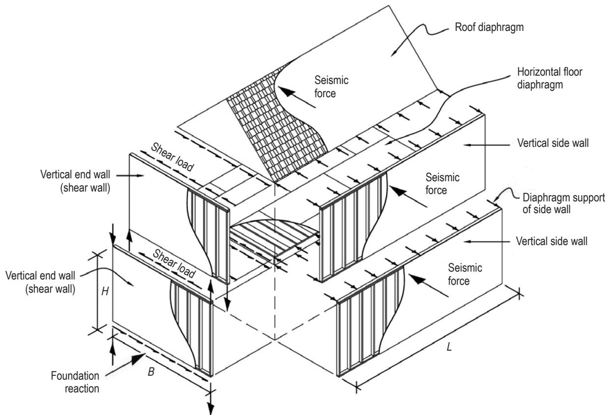
**Figure 1-1.** Wood light-frame building with load path illustrated (FEMA 2006).
