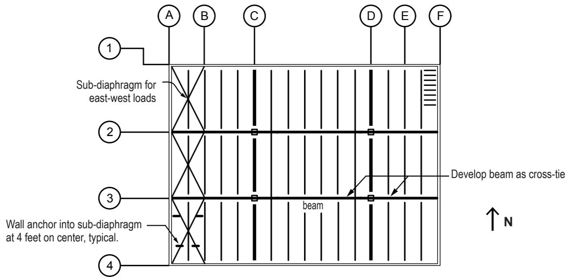
**Figure 3-7.** Plan of roof diaphragm with subdiaphragms for concrete or masonry wall seismic anchorage for loading in the east-west direction.
