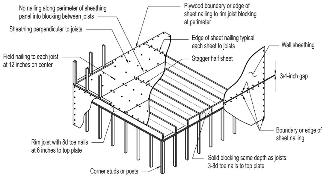
(a) Unblocked wood light-frame diaphragm (FEMA 2006).
