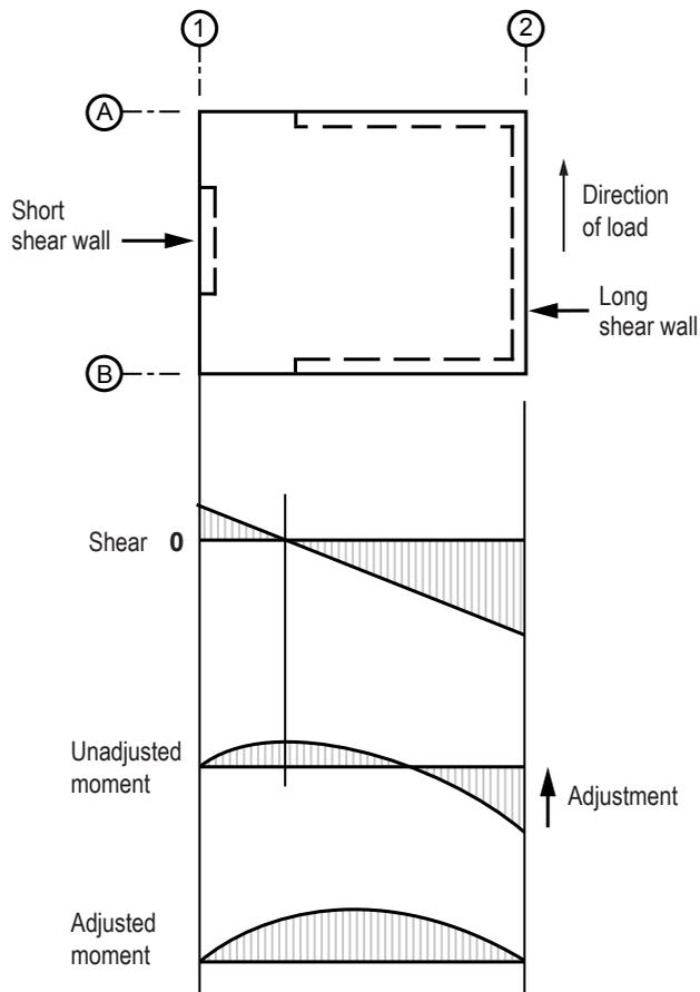
**Figure 6-1.** Plan view of a rigid diaphragm supported on shear walls of differing stiffness.
