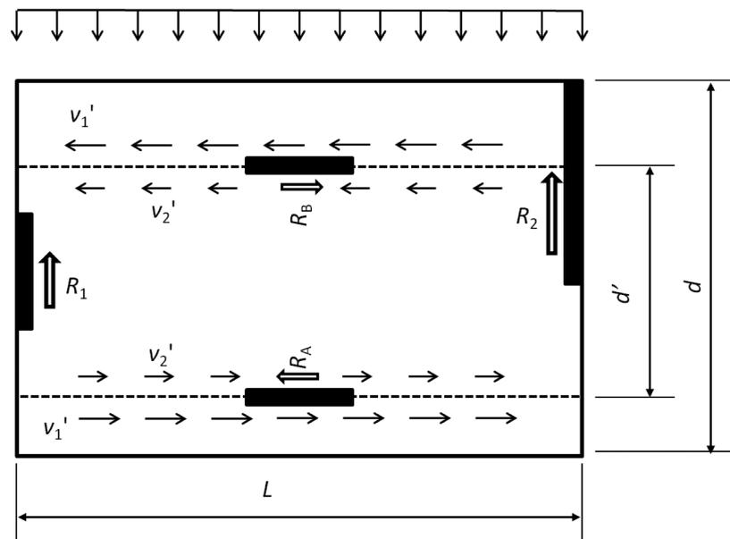
**Figure 6-2.** Plan view of diaphragm with shear walls inset from the diaphragm perimeter. Dimension  $d$  is the full dimension of the diaphragm, whereas dimension  $d'$  is the dimension between shear walls resisting torsion
