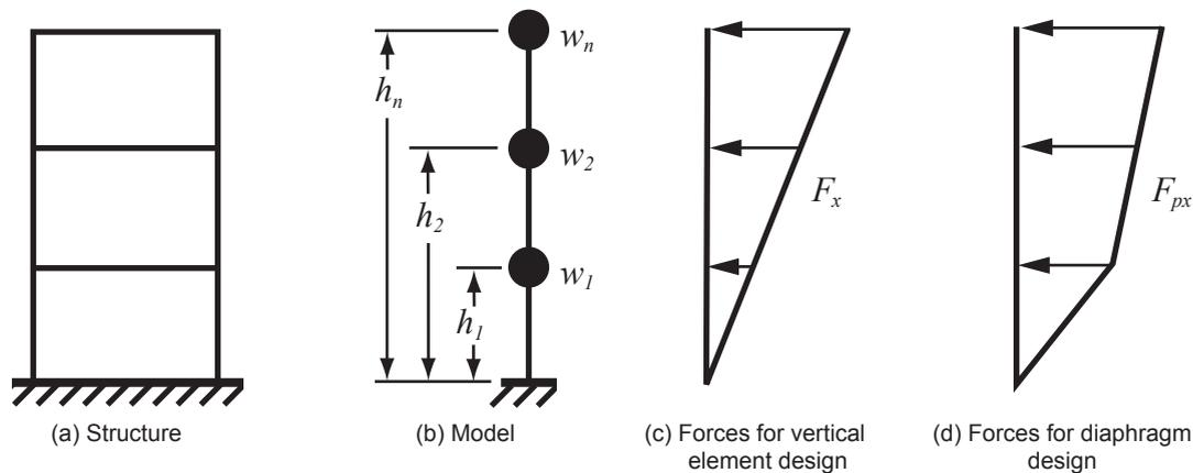
**Figure 4-6.** Vertical distribution of seismic forces based on ASCE 7 equivalent static force design procedures.
