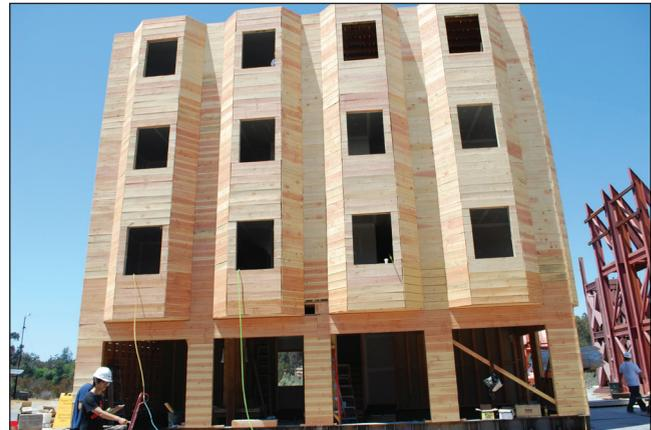
**Figure 4-3.** Soft ground story building, representing older San Francisco apartment building conditions, tested on the University of California, San Diego shake table.
