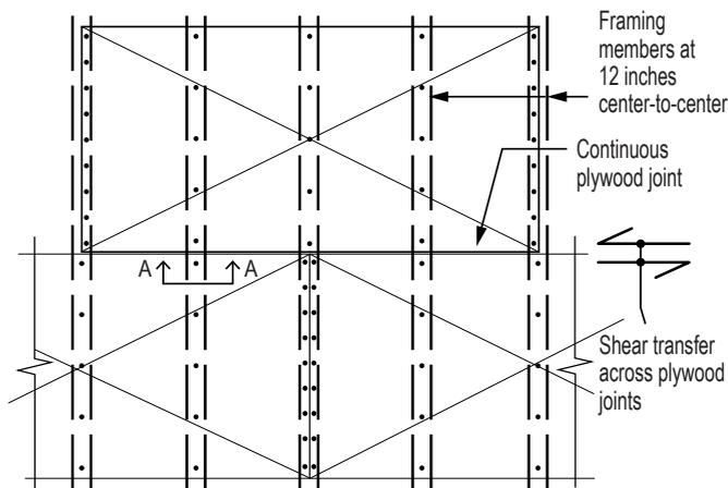
(a) Unblocked wood light-frame diaphragm shear transfer across a continuous sheathing joint.
