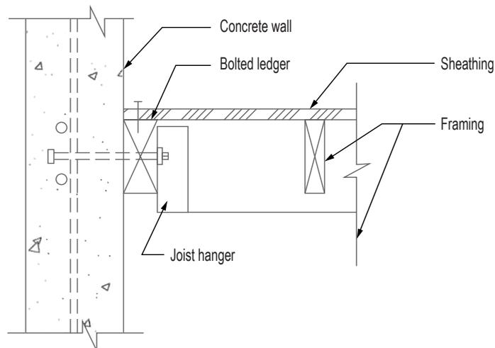
**Figure 3-9.** Inadequate concrete wall to wood light-frame diaphragm connection, lacking wall anchor capable of resisting direct tension.
