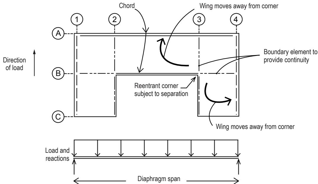
Figure 5-2. Plan view of diaphragm showing reentrant corner and potential seismic response.
