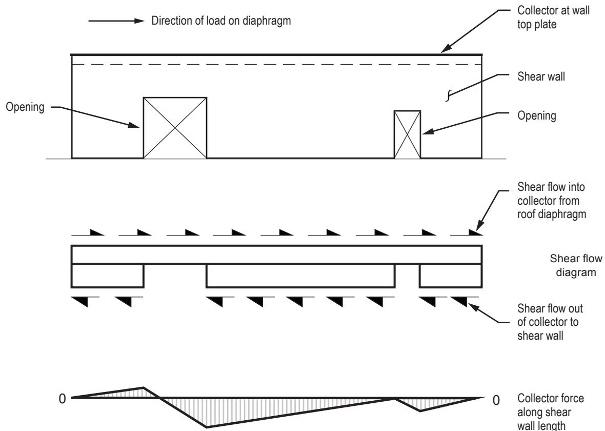
**Figure 3-5.** Wall top plate acting as collector boundary element. The diagram below the wall shows the variation in collector force along the collector length.
