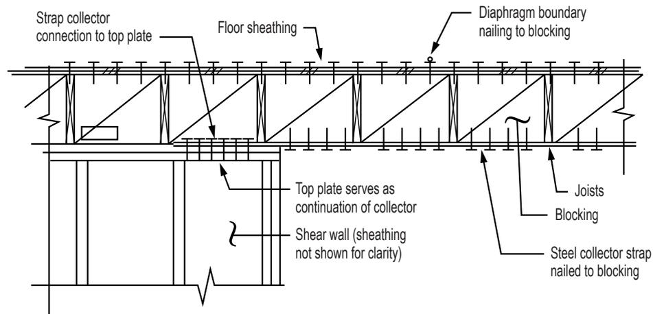
**Figure 7-2.** Steel strap and blocking providing a boundary member perpendicular to framing direction.
