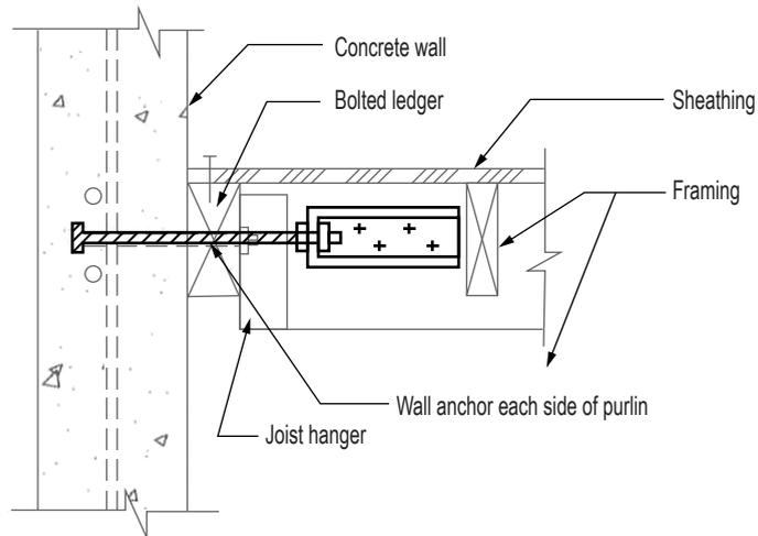
**Figure 3-8.** Concrete wall anchor to wood light-frame diaphragm or sub-diaphragm.
