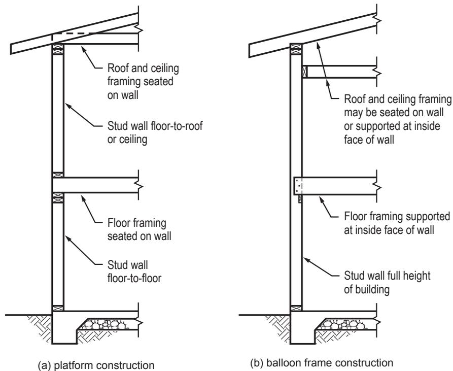
Figure 1-6. Typical wall sections.
