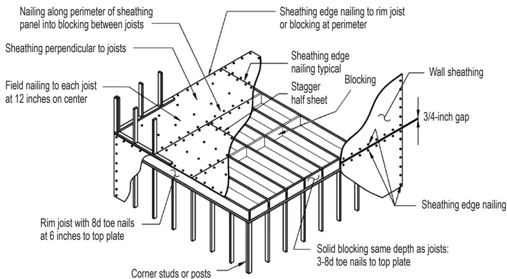
(b) Blocked wood light-frame diaphragm (FEMA 2006).
