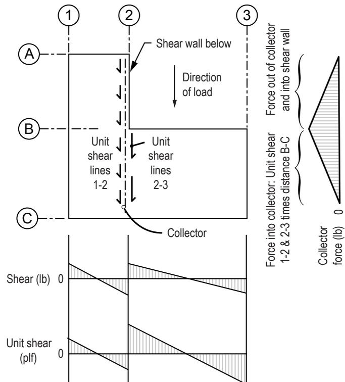
**Figure 5-1.** Plan view of diaphragm with its collector force diagrams.
