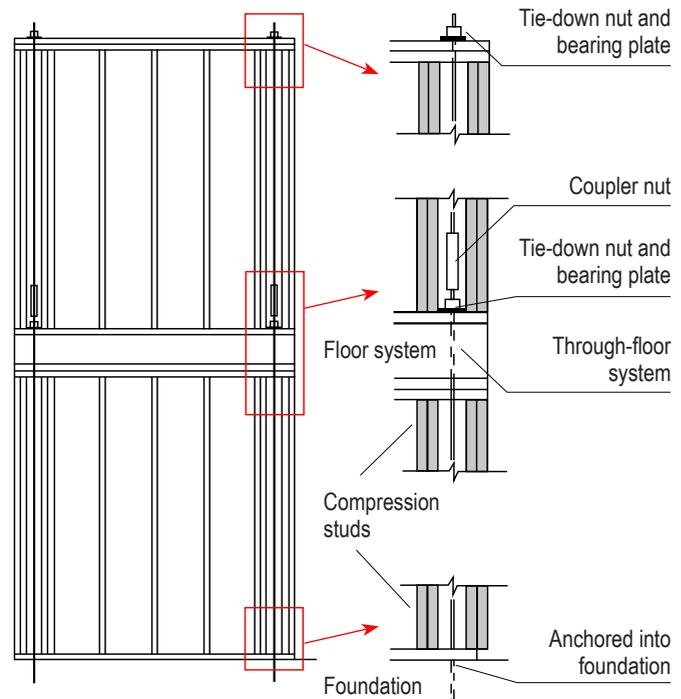
**Figure 4-7.** Elevation view of two-stories of a typical mid-rise wood light-frame shear wall stack.
