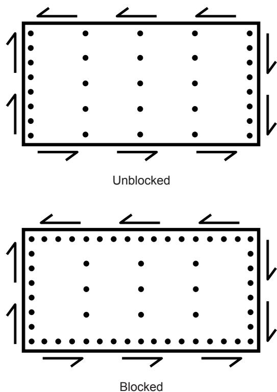
Figure 8-1. Shear transfer in wood structural panels.
