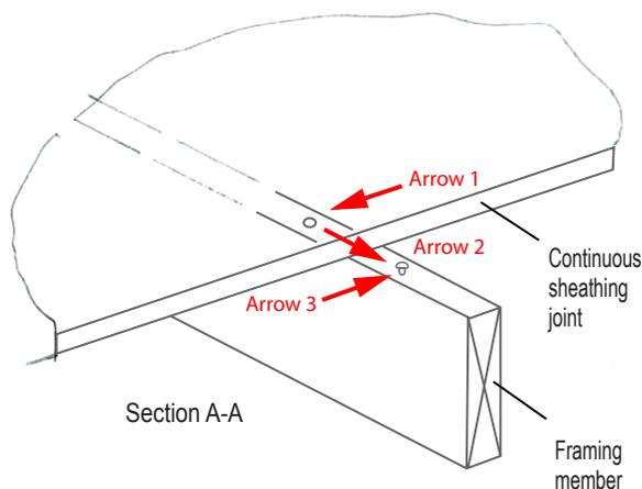
(b) Close-up of Section A-A. The shear force is transferred out of one sheathing panel and into the framing member at one fastener (Arrow 1), transferred horizontally through the framing member to the other fastener (Arrow 2), and then transferred through the fastener to the adjacent sheathing panel (Arrow 3).
