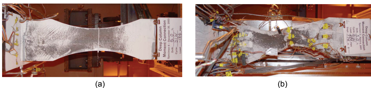
Figure 2-5 Results from connection tests of RBS beams with deep columns: (a) balanced panel zone design; (b) strong panel zone design (Ricles et al., 2004a).
