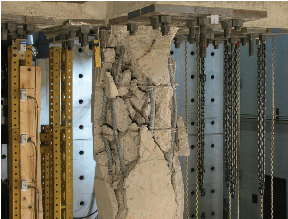
Figure 3-4 Column specimen PU8 tested to axial failure (Courtesy of NEES Grand Challenge).
